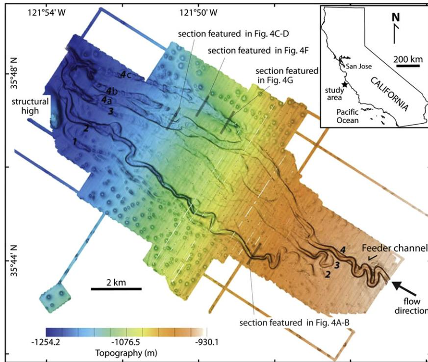
**Figure 3.** Multibeam bathymetry of the Lucia Chica channel system acquired with the Monterey Bay Aquarium Research Institute's (MBARI) Autonomous Underwater Vehicle (AUV). The inset map shows the approximate location of the dataset off the Pacific Coast of California. The channels of interest are numbered based on relative age, with 1 the oldest and 4 the youngest (modified from Maier et al., 2011).
